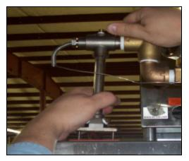
Lifting the rinse injector to make room
